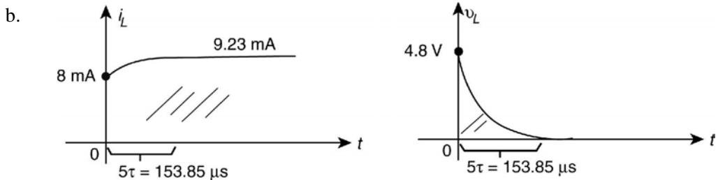
16. a.  $I_i = -8 \text{ mA}, I_f = 9.23 \text{ mA}, \tau = \frac{L}{R} = \frac{120 \text{ mH}}{3.9 \text{ k}\Omega} = 30.77 \mu\text{s}$
