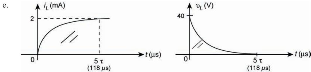
12. a.  $\tau = \frac{L}{R} = \frac{4.7 \text{ mH}}{2.2 \text{ k}\Omega} = 2.14 \mu\text{s}$
