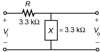
For frequencies near  $f_p$ ,  $X_L \gg R_\ell$  and  $Z_L = R_\ell + jX_L \cong X_L$  and  $X = X_L \parallel X_C$ .
