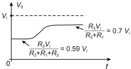
$$\mathbf{A}_v = \frac{\mathbf{V}_o}{\mathbf{V}_i} = \frac{R_3}{R_3 + R_1 + R_2 \parallel X_C \angle -90^\circ}$$
