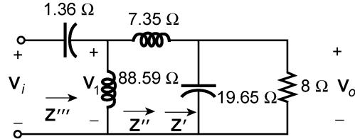
$$\mathbf{Z}' = \overbrace{7.41 \Omega}^{\text{Z}'} \angle -22.15^\circ$$
