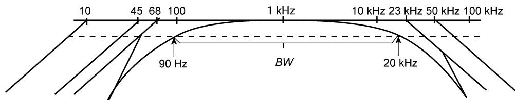
$50 \text{ kHz}$  vs  $23 \text{ kHz} \rightarrow$  drop about  $1 \text{ dB}$  at  $23 \text{ kHz}$  due to  $50 \text{ kHz}$  break.
