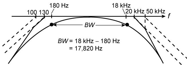
Proximity of 100 Hz to 130 Hz will raise lower cutoff frequency above 130 Hz:
