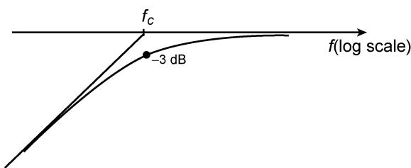
c.  $f = \frac{1}{2}f_c$ :  $A_{v_{dB}} = 20 \log_{10} \frac{1}{\sqrt{1+(f_c/f)^2}} = 20 \log_{10} \frac{1}{\sqrt{1+(2)^2}} = -7 \text{ dB}$
