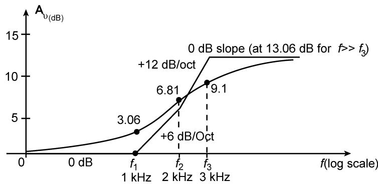
55.  $\frac{j\omega}{1000} = j\frac{2\pi f}{1000} = j\frac{f}{1000} = j\frac{f}{159.16 \text{ Hz}}, \frac{j\omega}{5000} = j\frac{f}{795.78 \text{ Hz}}$
