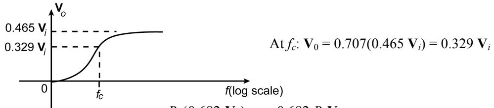
$$\text{At } f_c: V_o = 0.707(0.465 \text{ V}_i) = 0.329 \text{ V}_i$$
