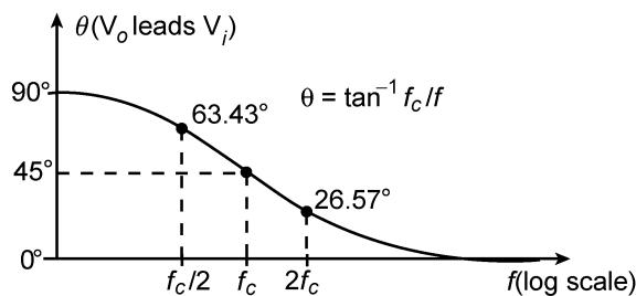
39. a.  $f_c = \frac{1}{2\pi RC} = \frac{1}{2\pi(6.8 \text{ k}\Omega \parallel 12 \text{ k}\Omega)0.02 \mu\text{F}} = \frac{1}{2\pi(4.34 \text{ k}\Omega)(0.02 \mu\text{F})} = 1.83 \text{ kHz}$
