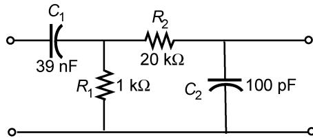
$$\text{Center frequency} = 4 \text{ kHz} + \frac{80 \text{ kHz} - 4 \text{ kHz}}{2} = 42 \text{ kHz}$$
