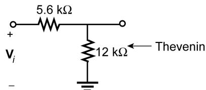
$$V_{Th} = \frac{12 \text{ k}\Omega V_i}{12 \text{ k}\Omega + 5.6 \text{ k}\Omega} = 0.682 V_i$$
