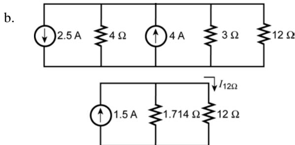
$$I_{12\Omega} = \frac{(1.714 \Omega)(1.5 \text{ A})}{1.714 \Omega + 12 \Omega} = \mathbf{0.19 \text{ A}}$$
